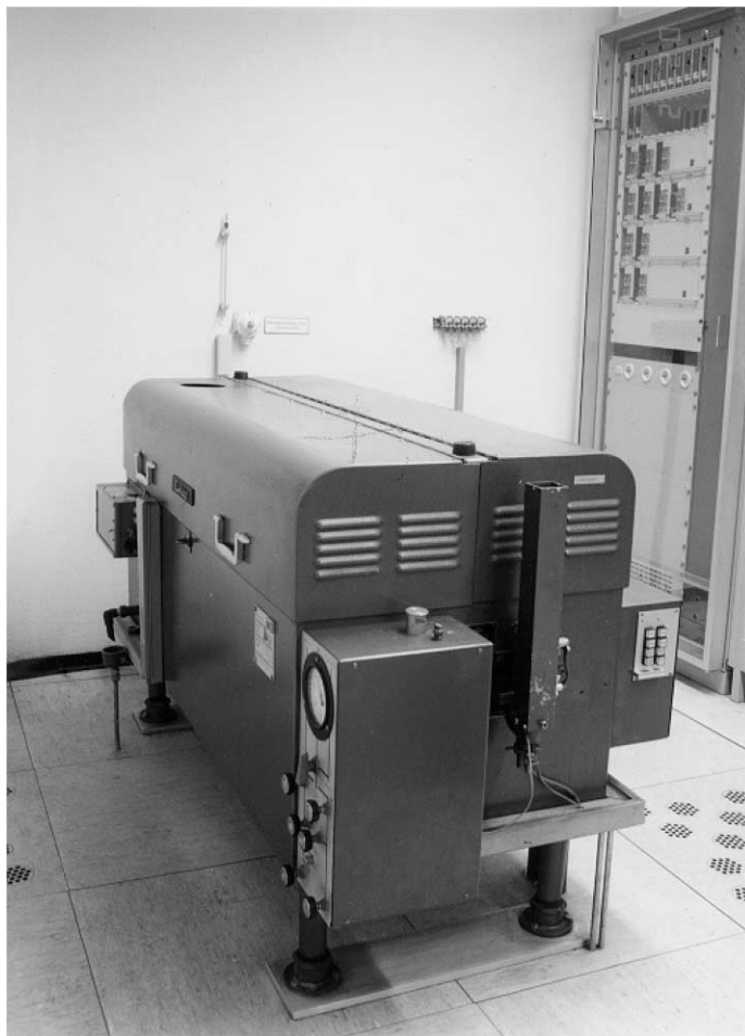
Fig. 1. The Thomas–Cambridge calorimeter.
